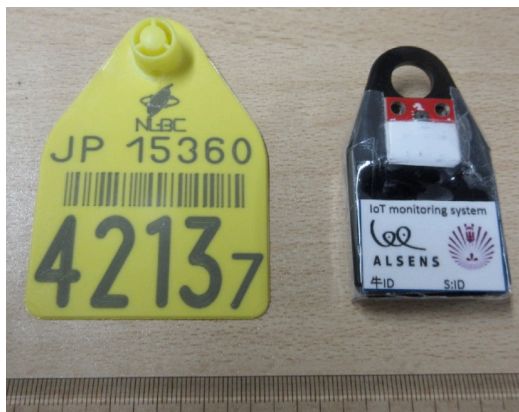
Fig. 1 Photograph of the proposed ear tag
